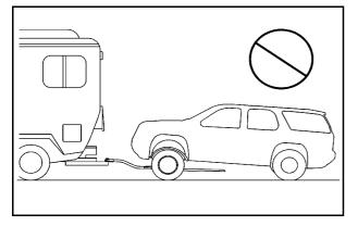
*Notice:* If a two-wheel drive vehicle or a four-wheel drive vehicle with a single speed automatic transfer case is towed with the rear wheels on the ground, the transmission could be damaged. The repairs would not be covered by the vehicle warranty. Never tow the vehicle with the rear wheels on the ground.
